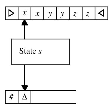
Here we have some memory (in the form of a "work tape") as well as the input.
