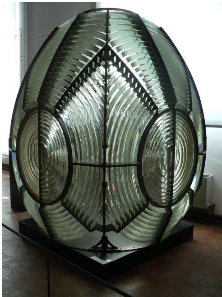
First-order rotating catadioptric Fresnel lens, dated 1870, displayed at the Musée national de la Marine, Paris.
