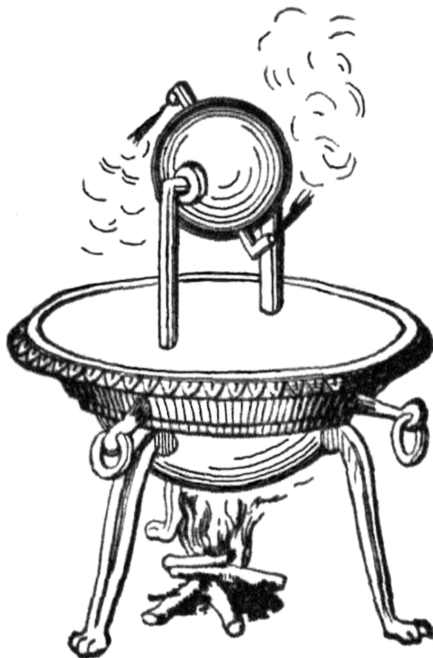
Hero's Aeolipile Engine
