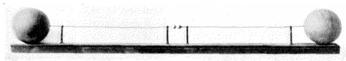
The first spark gap oscillator built by Heinrich Hertz around 1886
