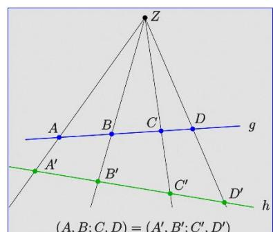
One of the most important principles of *Projective Geometry* is the *duality principle* (called the *reciprocity law* by PONCELET): In the plane, for example, points and straight lines are dual objects to each other. For a proposition about points and straight lines, one obtains the corresponding dual proposition by interchanging the terms.
